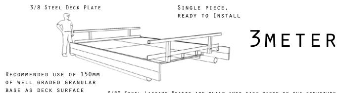
3/8" Steel Lifting Points are build into each piece of the structure
